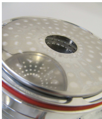
Fig 1. Powder collected on a stage of the Anderson Cascade Impactor.
